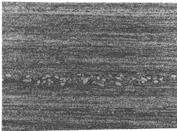
Figure 3 Etched section of as-extruded Cu-5 wt % Nb-2.5 wt % Sn parallel to the extrusion condition, showing inhomogeneous microstructure.
