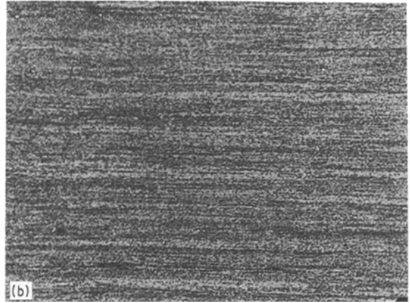
Figure 2 Etched sections of as-extruded Cu-5 wt % Nb-2.5 wt % Sn (a) Section perpendicular to the extrusion direction (b) Section parallel to the extrusion direction.
